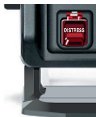
Distresstaste am DSC-Controller
